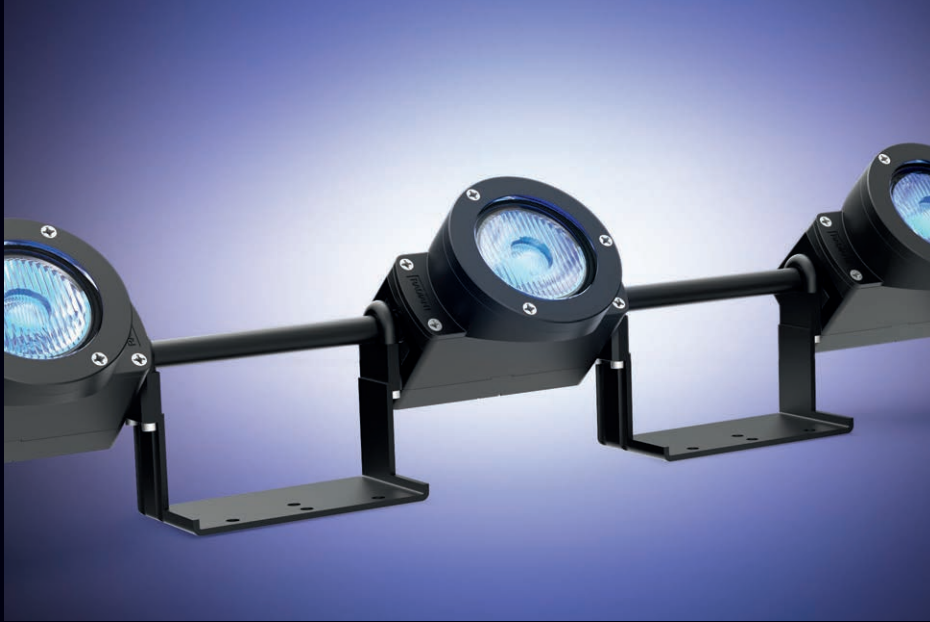
3D LED Flex 40 System IP66 RGBW - 200 mm module pitch Each module is individually addressable via DMX
